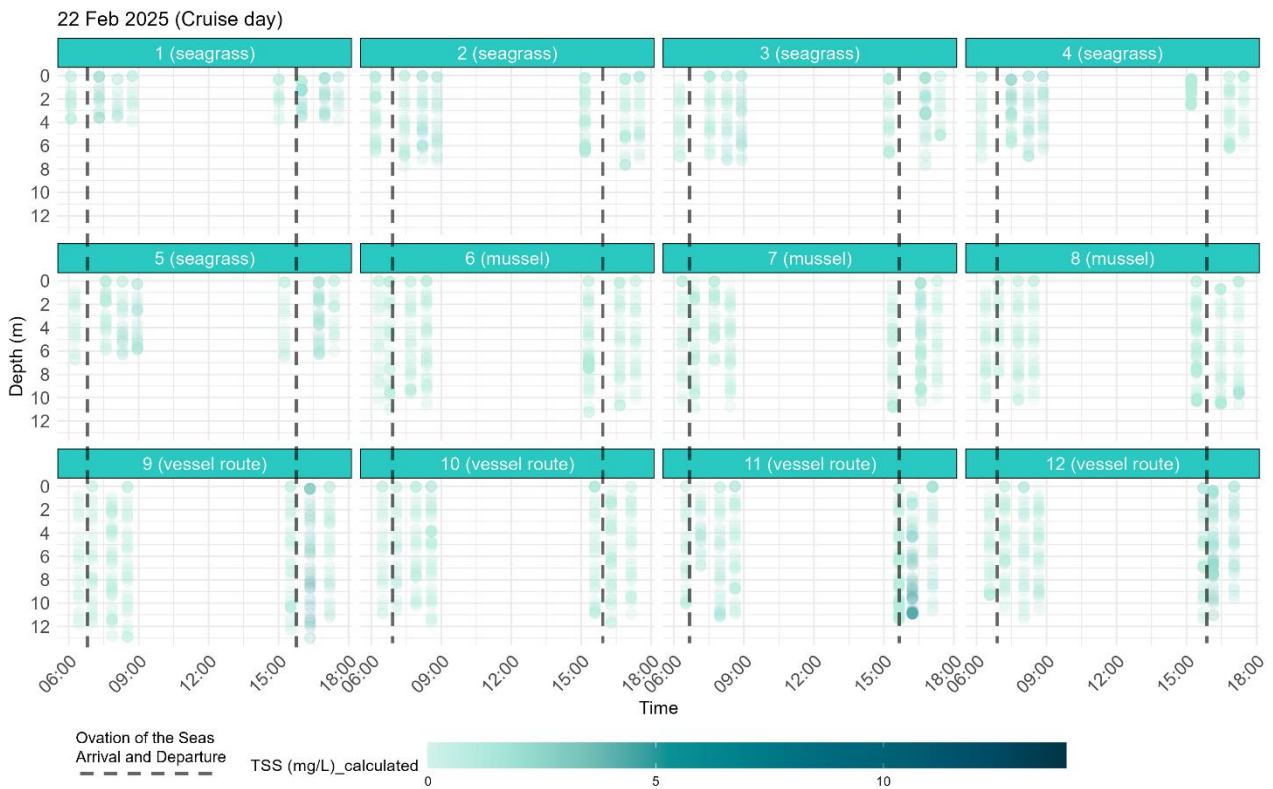
Figure 3-19 Calculated TSS (mg/L) concentrations by water depth and time. Plot shows results for the day of the cruise vessel visit with arrival and departure times shown with dotted lines.
