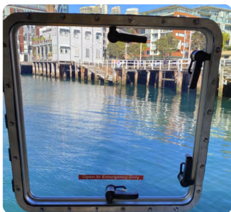
ESCAPE HATCH ON PV SEVER
