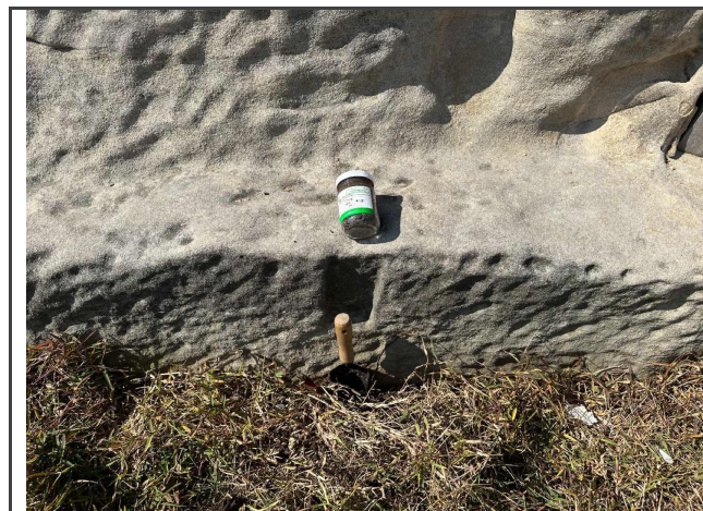
PHOTO: 4 LOCATION: External, GF Perimeter South east of the lighthouse - within the run off MATERIAL: Soil (heavy metal contaminants) RESULT: Refer to Sampling Register
