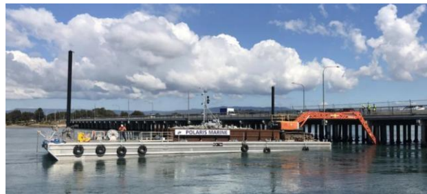
Figure 5: Typical 30m transport barge
